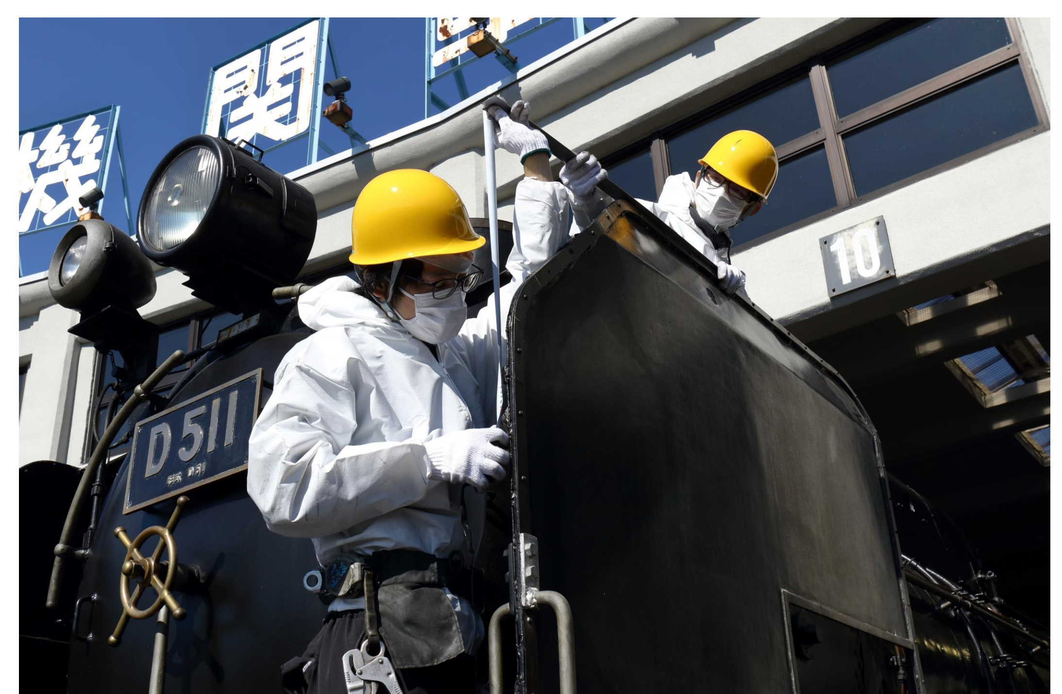
Measuring and 3D modelling the deflector of Type D51 at the Kyoto Railway Museum.
