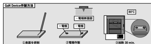
図1 GaN LED Wafer Device の作製手順
