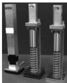
図 1 Previous leg (left) and the new legs with a spring (middle and right)
