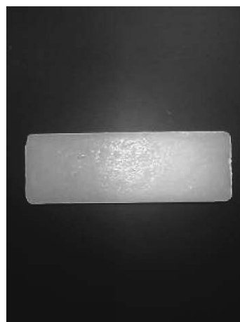
Figure 1 Photograph of ESO-PBS hybrid (50 : 50 wt%).
